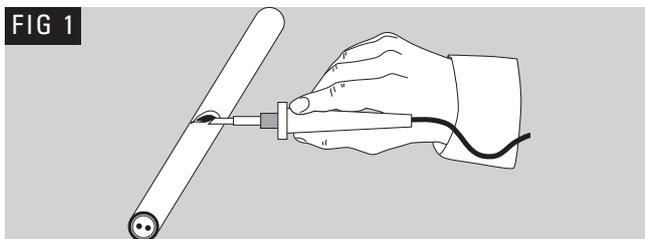
For minor repairs, the LSF material adjacent to the damage can be re-moulded. This is achieved by using an electric soldering iron or a hot knife to melt the material and redistribute it (Fig 1). The soldering iron is the most convenient, as it remains hot in use. More extensive damage will necessitate the use of a larger soldering iron.
