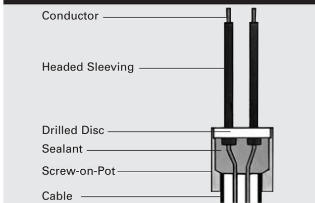
Earth Tail seals are available incorporating a 150mm length of protective conductor identified by green/yellow striped sleeving. The dimensions of screw-on pots are shown below.
