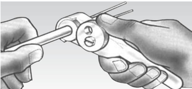
Engage the ratchet wheel into the knurled section of the pot and maintain this contact with thumb or finger as appropriate. Applying forward pressure and a cranking action, screw the pot squarely onto the cable.
