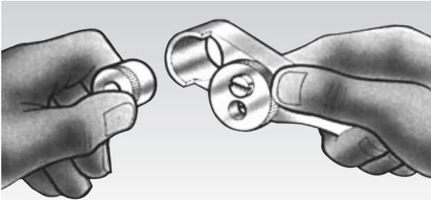
Insert the seal pot open end first into the tool recess.
