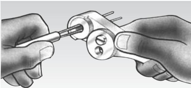
Feed the exposed conductors through the seal pot until the cable sheath is in contact with the self cutting thread of the pot.
