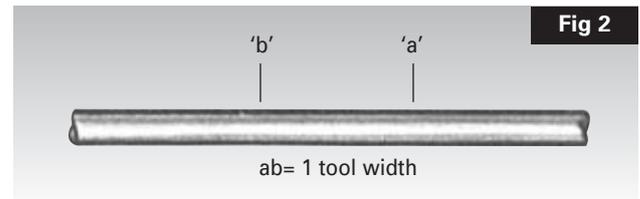
Having previously marked the sheath at the point where stripping is to stop (point 'a' in Fig. 2), add a second pencil mark one tool width further along the sheath (point 'b' in Fig. 2) to indicate the position for location of the pliers. When using tool reference ZSU or ZSUS insert the cable into the tool as far as the face of the cutting wheel (Fig. 3). Tighten knurled screw until the tool can just support its own weight in a horizontal position.
