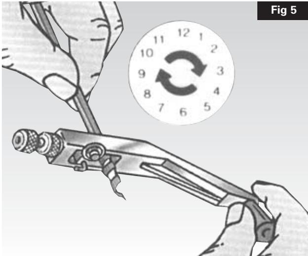
Rotate tool in a clockwise direction applying slight pressure in the direction of stripping until in the case of the ZSU and ZSUS Strippers sufficient swarf has been formed to allow it to be bent round the adjacent post (Fig. 5 and 6). This will prevent the tool snagging the swarf. Once stripping has commenced, all 3 rotary stripping tools will propel themselves along the cable.
