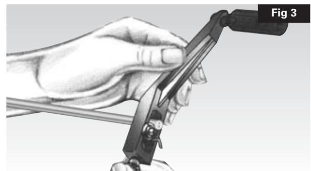
When using the Joistripper set the guide block as follows:
