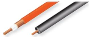
*Mi Cable with 3x25 mm<sup>2</sup> has diameter of 18.2 mm. A typical polymeric equivalent 3 core 25 mm<sup>2</sup> cable is 27.4 mm diameter (50% larger than the MI equivalent.) Remember, it is typical for conductors on polymeric cables to be over-sized to protect the cable from harmonic loads, overheating and premature aging.*
